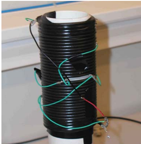
Figure 17. RG-58 transmission line test transformer.
