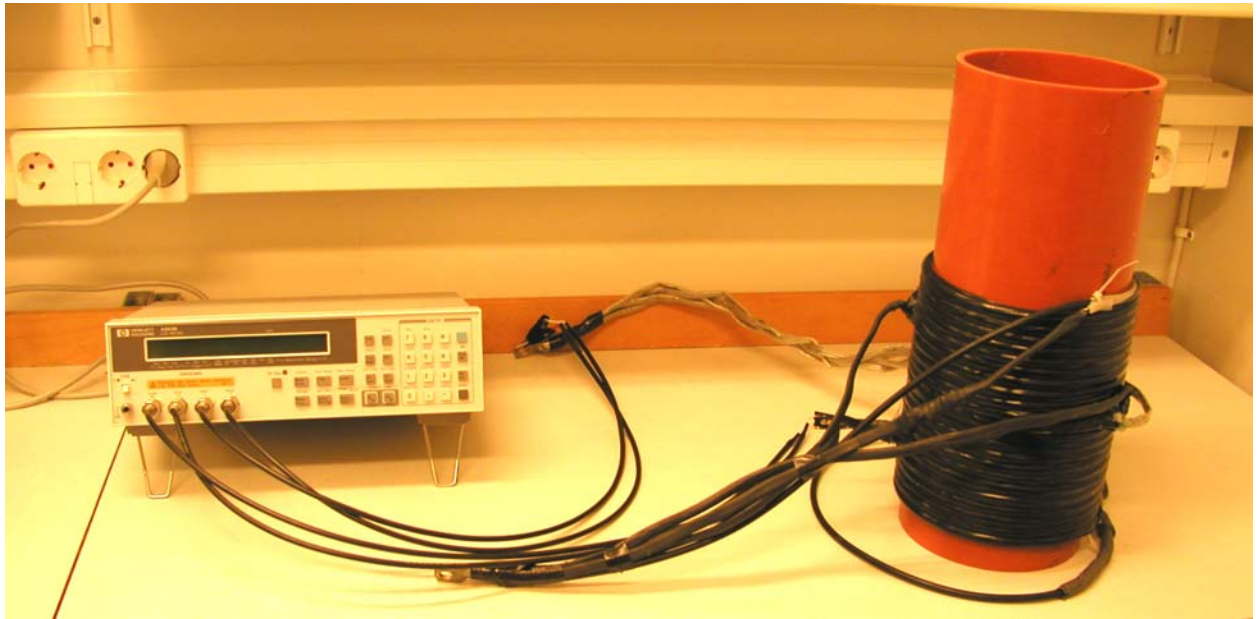
Figure 24. Inductance measurement of semicon transformer.
