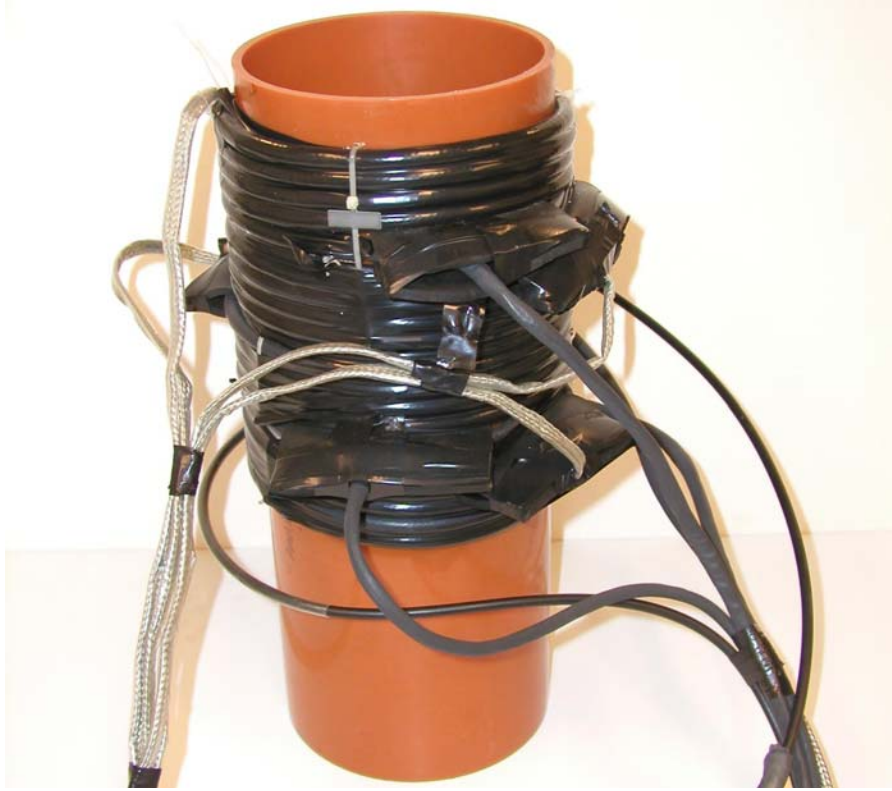
Figure 48. Modified transformer with rubber insulated terminals.
